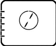
Warm air heated by the rear heater is evenly distributed throughout the oven rapidly by means of the fan. It is suitable for cooking your meals in different rack levels and preheating is not required in most cases. Suitable for cooking with multi trays.
