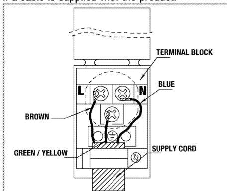
2. **For single-phase connection**, connect the wires as identified below:
