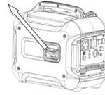
Push the choke knob in to the original position.
