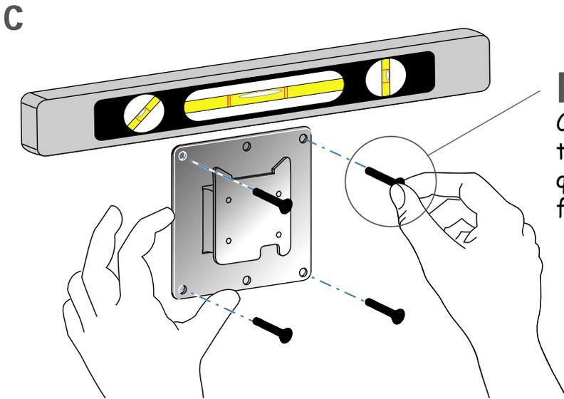
**NOTE:** Fasteners are not supplied. Consult a qualified construction professional to determine the appropriate type and quantity of mounting fasteners required for your application.
