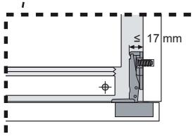
**Note:** Installation step for 2, screws for connecting top plastic part should not be screwed very hard, because of moving the plastic part easily left or right side.
