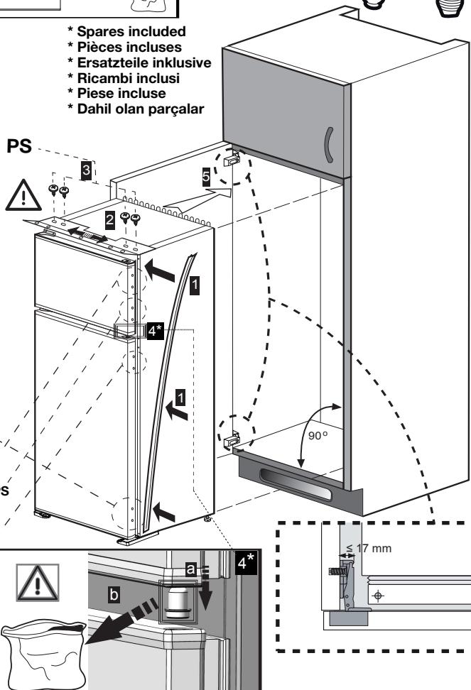
**Note:** Installation step for 2, screws for connecting top plastic part should not be screwed very hard, because of moving the plastic part easily left or right side. **Installation step for 4\* - only for Italy models.**
