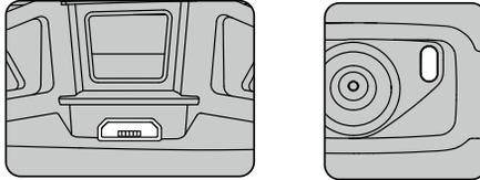
The Aircraft Status Indicator blinks blue slowly during charging. The battery is fully charged when the Aircraft Status Indicator turns solid blue. Detach the USB adapter when the battery is fully charged.
