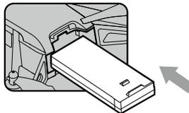
To remove the battery pull it out from the aircraft.
