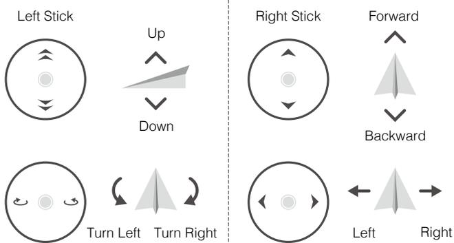
The figure below explains how to use each virtual joystick, using Mode 2 as an example.
