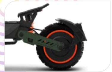
Motore Brushless 500 W, 23.5 Nm, KERS, Peak Power 2000 W
