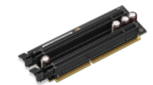
ThinkStation PCIe x16 to 2 PCIe x8 Riser Card
