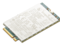
ThinkPad Foxconn SDX61 5G Sub6 PCIE M.2 3052 WWAN module for T14 G7 4XC1V64420
