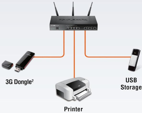
Supports one (DSR-250N) or two (DSR-1000AC) USB 2.0 devices to extend functionality.
