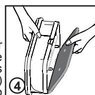
5. Refit the front cover ensuring it is in the correct way (as indicated by the arrow) and pushed firmly into place. Lock the two levers by turning them clockwise
