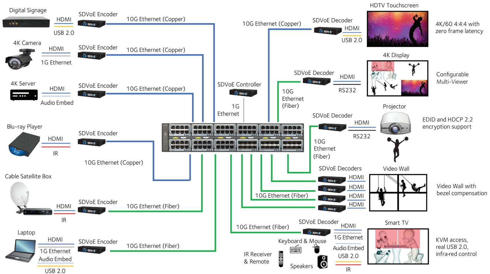
To take the complexity out of your AV-over-IP deployment, NETGEAR created M4300 switches that are preconfigured for easy, true AV and multicast Zero Touch network configuration. Namely, IGMP Snooping, IGMP Fast Leave, IGMP Querier are already enabled for the default VLAN 1 that all your devices will automatically use. Connect your encoder and decoder devices, and power on the switch – it just works!
