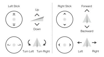
The figure below explains how to use each virtual joystick, using Mode 2 as an example.
